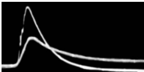
Fig. 5. Impulse from laser irradiation of a surface in air (lower trace) and underwater (upper trace)
