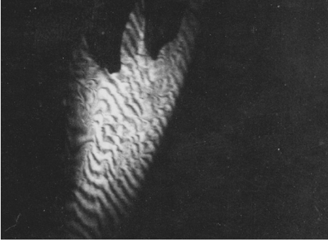
Fig. 2. Double-exposure hologram of the leg of the Donatello painted wood carving revealing hidden cracks.
