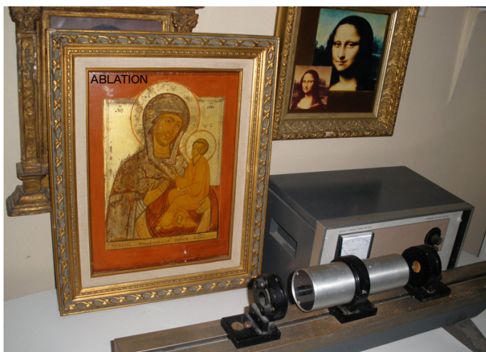
Fig. 7. 1962 Hughes Company ruby laser copy of Theodore Maiman's original laser used by George Stout in the first radiation-divestment cleaning of a painting (Serbian Icon shown).
